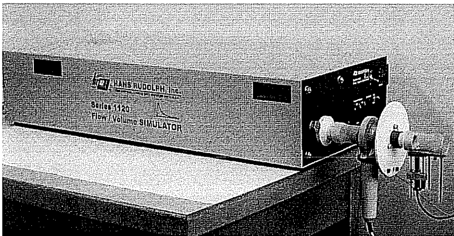
Fig. 1 The Flow / Volume Simulator with attached PTB-FM and temperature sensor
